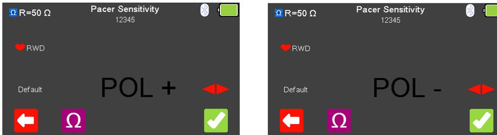
The Polarity of the Pacer Sensitivity can be selected using the
