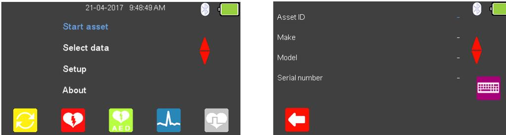
The Asset ID, Make, Model and Serial Number of the appliance under test can be added, to exit without saving select
