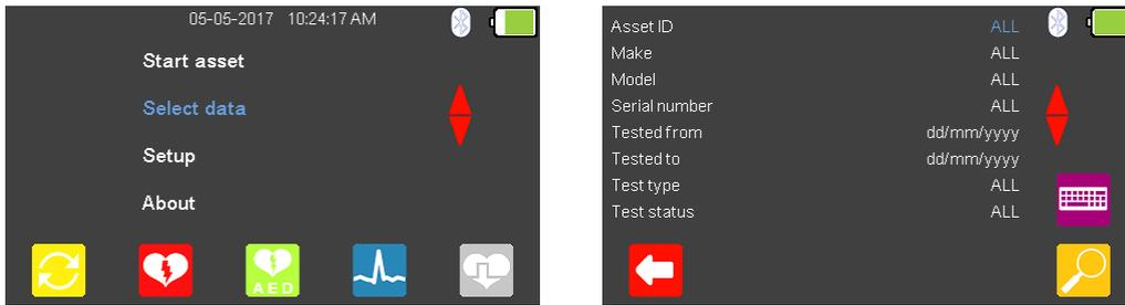
From the Main Menu, use the arrow keys to highlight Select data and select the (return) key to enter the asset menu. The arrow keys can be used to highlight the item to be used in the search criteria. The search criteria can be either changed using the keyboard or using the arrow keys, where applicable (note the Bluetooth scanner can be used to input the Asset ID). Select (F5) to display the results.
