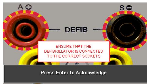
To enter the AED Pulse mode, you have to accept the connections warning using the ↵ (return) key, - the red and black 4mm defibrillator terminals are highlighted with a flashing red / yellow image.
