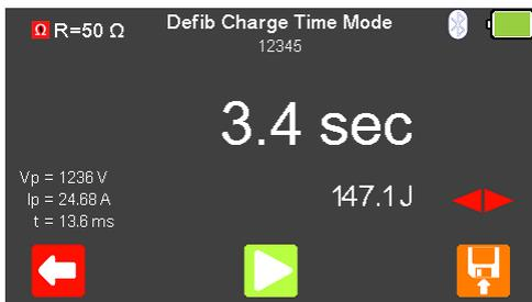
To accurately measure charge time the defibrillator charge must be initiated at exactly the same time as
