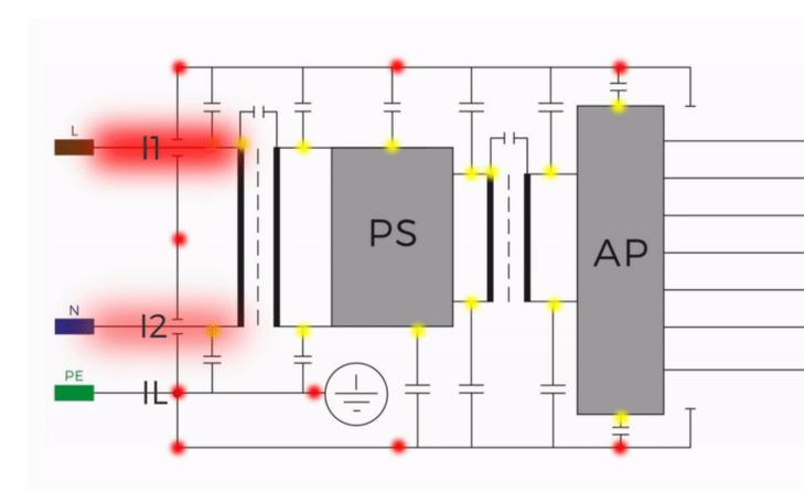
Earth leakage (IL) can be expressed as: I1 (L current) – I2 (N current)
