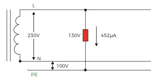
Figure 1: Potential difference and leakage currents on TN and Non-TN systems
